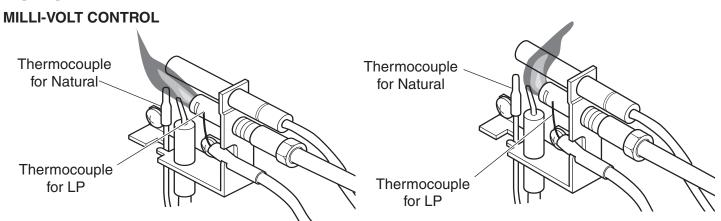
Figure 17 - Correct Appearance of Pilot Flame
